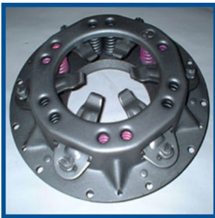
This is an original Model A style clutch pressure plate
