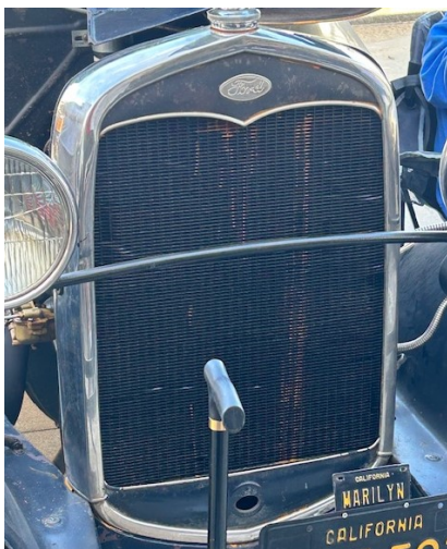
Telltale rusty signs of possible overheating problems.
