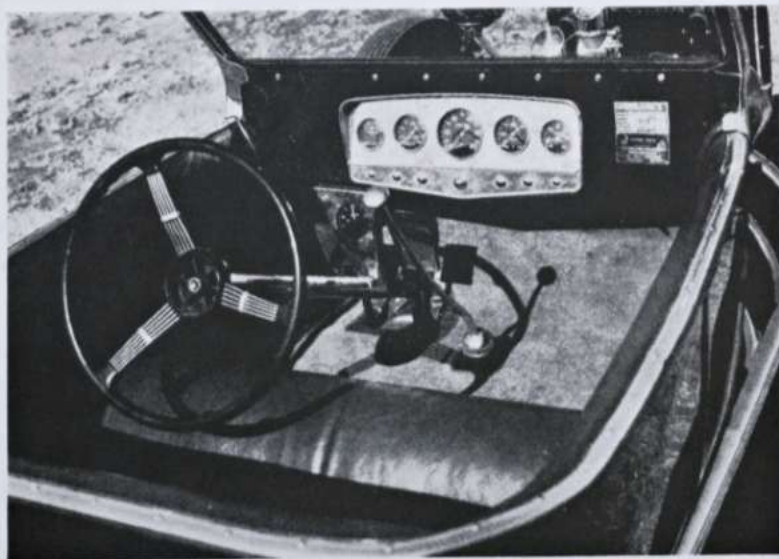
Interior has well-equipped dash with tachometer mounted in steering wheel bracket.
