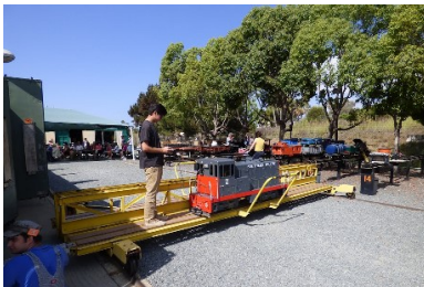
Remote control to bring trains out of storage bin and over to work station.
