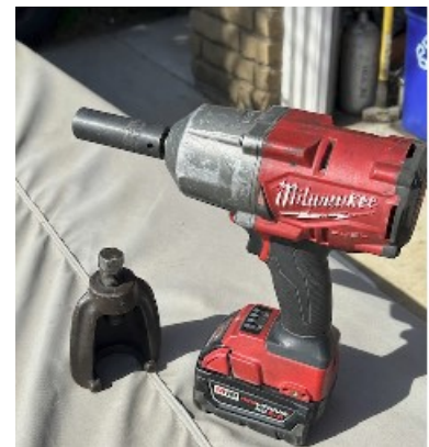
LATE model hub puller on left and SUPER handy battery powered impact gun on right.
