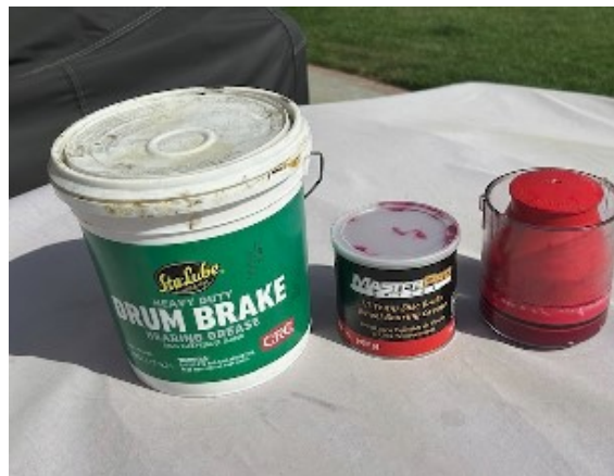
Several example of grease, with Wheel Bearing Packing tool on right
