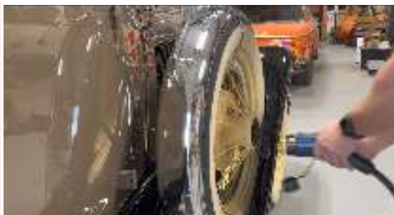
Where is the Charging Port? Behind the hubcap of the spare tire.
