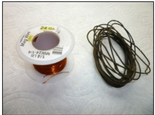
A roll of #24 gauge wire obtained from a local electronics store and the removed #20 gauge wire from one of the two fields.
