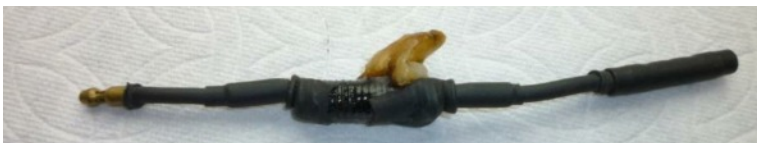
An ahooguh dropping resistor that burned out
